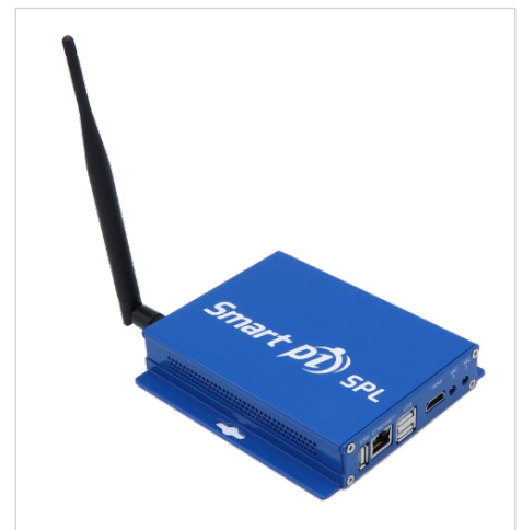
Smart pi fitted with wi-fi antenna
